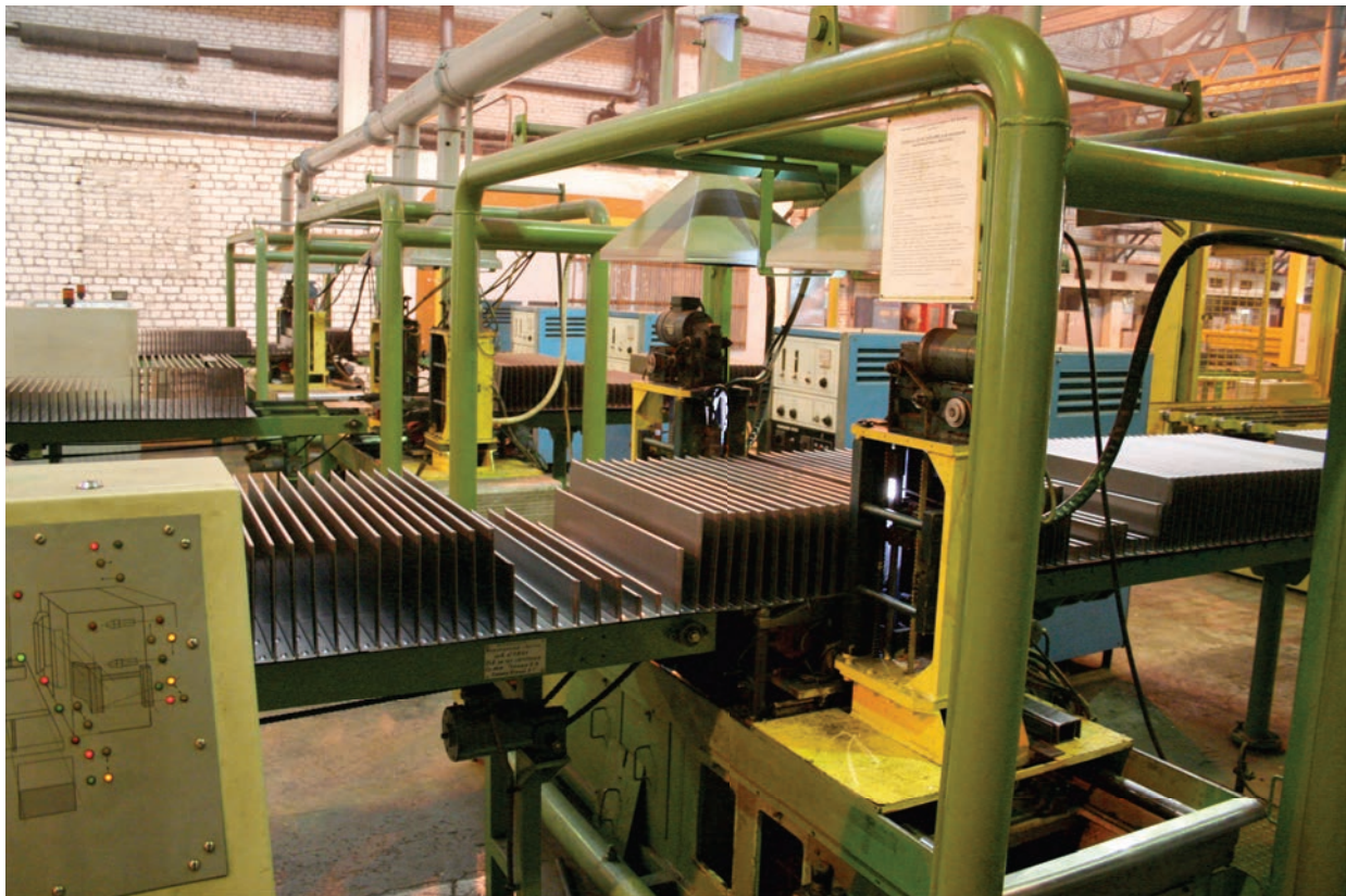
LINE FOR PLASMA WELDING OF CORRUGATED WALLS
